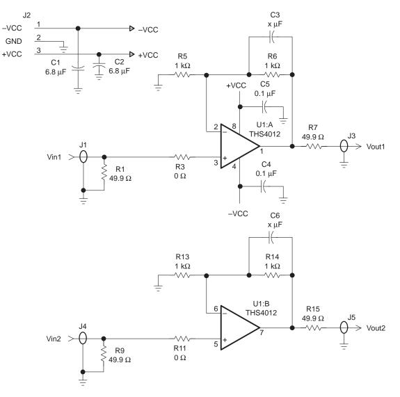
The gain of the EVM can easily be changed to support a particular application by simply changing the ratio of resistors R6 and R5 (channel 1) and R14 and R13 (channel 2) as described in the following equation:
